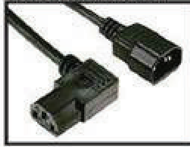
Item No. : E012018434_1.8M H05VV-F 3G 0.75MM 2 / 1.00MM 2 ,L=1.8M (VDE,UL,SAA APPROVAL)
