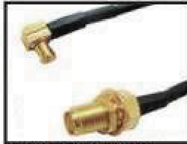
Item No. : Q116-043-012 RF CABLE ASS'Y ,MCX R/A- (RG174,200MM)-SMA(GOLD PLATED)
