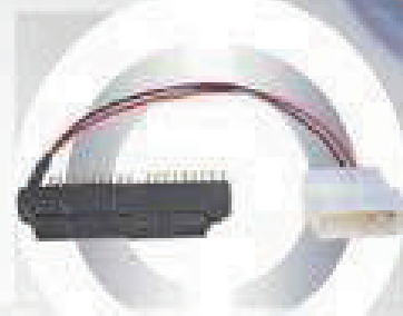
008307_0000A 3.5" TO 2.5" HDD ADAPTER
